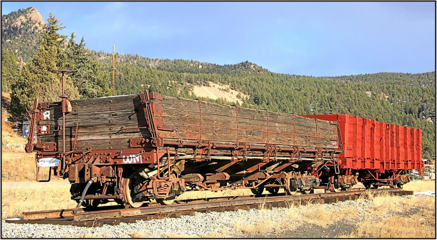
The D&RGW narrow gauge drop bottom gondola on display on the old South Park grade at Pine, Colorado, needing repairs and painting.
